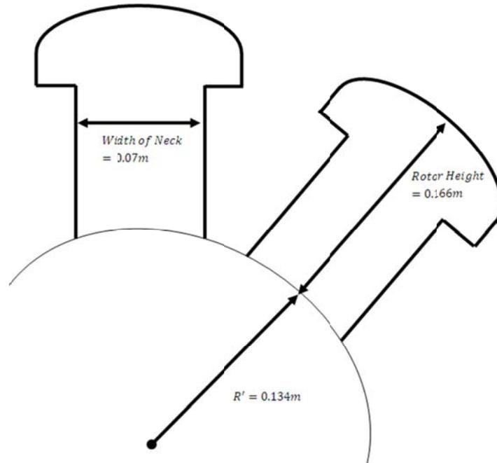
Figure 10 Width of the Rotor Shaft in Relation to Poles
