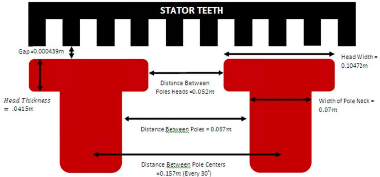
Figure 8 Dimensions of Rotor Poles
