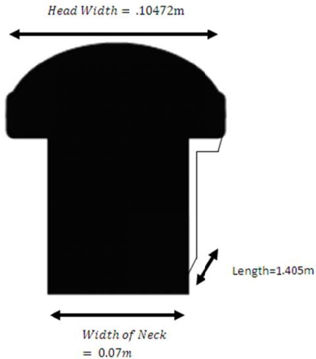
Figure 9 Rotor Pole Dimensions
