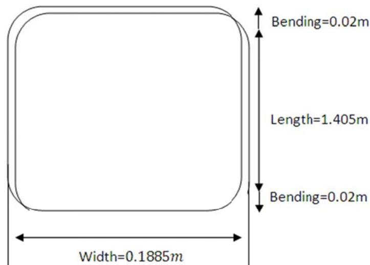
Figure 7 Coils Raps in Stator
