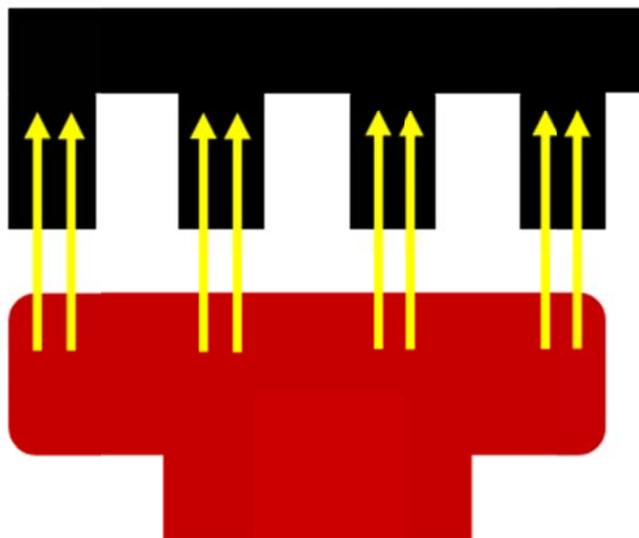
Figure 11 Flux off the Rotor into Stator
