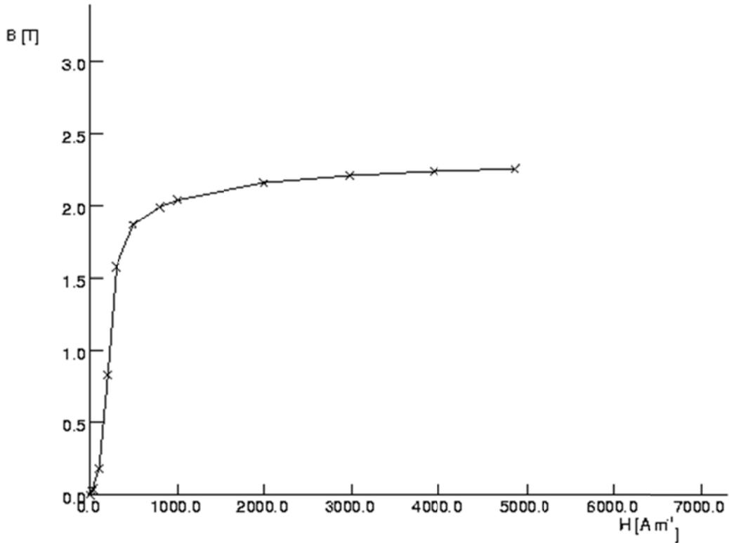
Figure 13 Magnetic characteristics of Vacoflux 50
