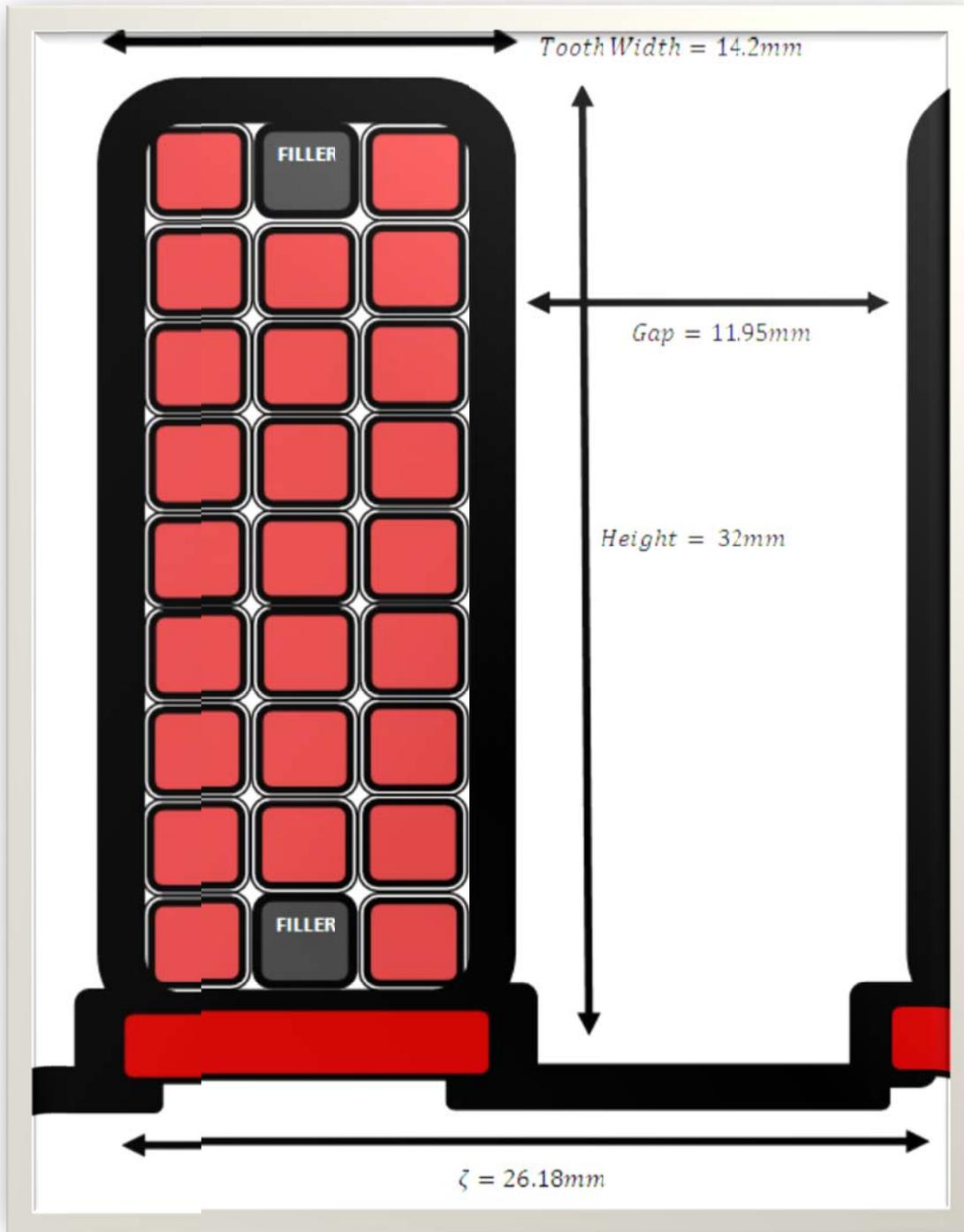
Figure 6 Conductor within Teeth Layout
