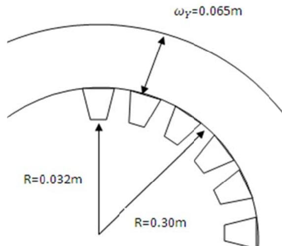
Figure 12 Yoke of Stator
