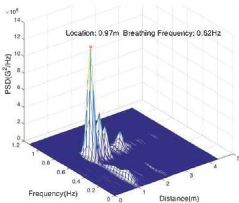
Figure 7 Location and frequency are determined by PSD
