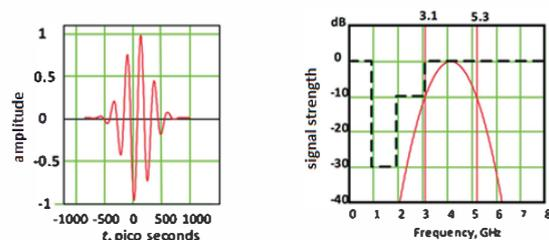
**Figure 1 (a)** Pulse transmitted by the radar **(b)** Transmit signal power spectrum
