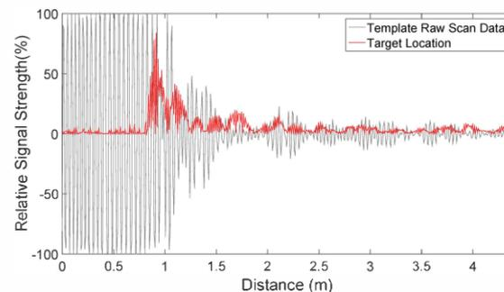
Figure 5 An example of the raw data acquired by the UWB radar from one scan
