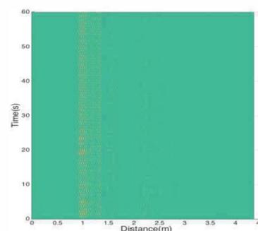
Figure 6 Two-dimensional signal plot after background removal and band pass filter
