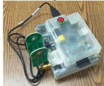
Figure 4 Experimental setup with UWB radar and an embedded processor
