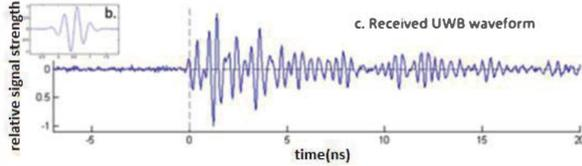
Figure 2 Comeback waveform sensed by the radar receiver
