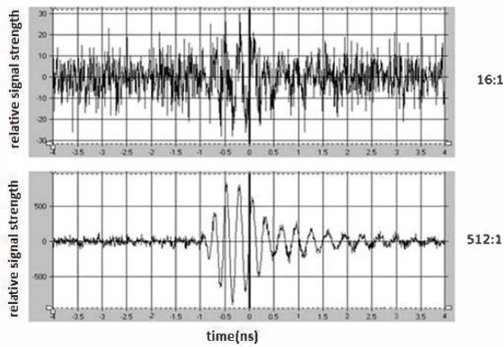
Figure 3 Received signal with different integrated ratio (16:1 means 16 received pulses are summed to form one scan and 512:1 means 512 received pulses are summed).
