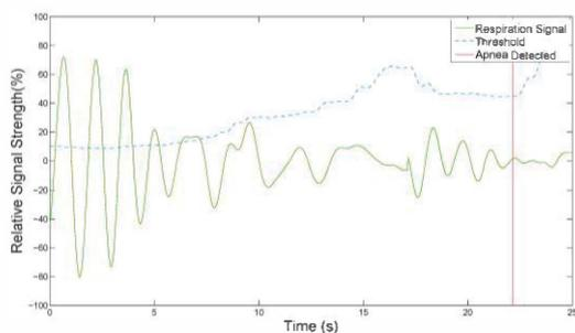
Figure 9 Apnea is reported if no breathing signal is above the threshold for 15 seconds
