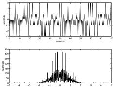
So, which is better? T-wide Hamming blip spectrum has lower power bandwidth (but higher null-to-null) bandwidth than the spectrum of a T-wide rectangular pulse.
