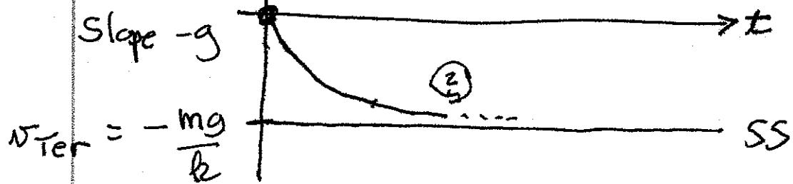
$\frac{dv}{dt} = 0$  when not falling faster - at  $v_{\text{terminal}}$
