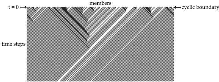
Fig. 2. The emergent behavior of the CA in Fig. 1 given a disordered initial condition of 200 members long played out for 100 progressions. The spatial dimension runs left to right; the temporal, top to bottom. The spatial dimension has cyclical boundary conditions.
