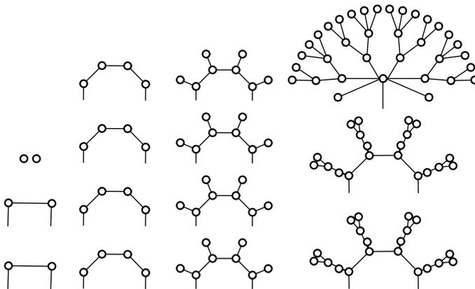
Fig. 8. State progression graphs for an eight-member 1D Ising system in isolation. Each community is symmetric; so, only half of each is shown.
